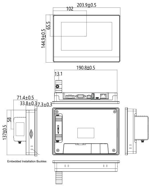
Panel Cutout of Embedded installation: 192mm\*138mm (+1.0/-0.0mm)
